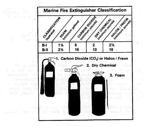
Boat fires also may be caused by electrical wiring (Class C). The current overloads the wire, gets it hot, and sets the insulation on fire. An extinguisher must be able to put out this fire without giving the user a shock. Use dry chemical, CO2, or Halon/Freon.
