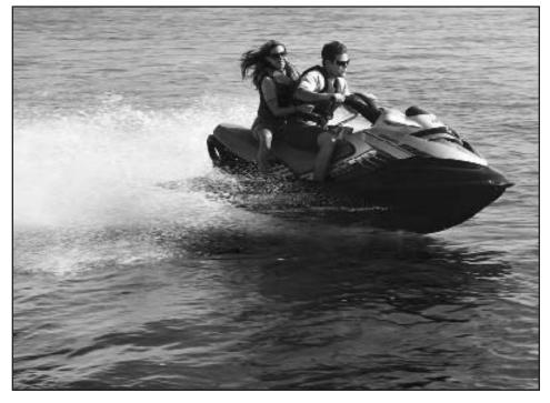
is turned right, the nozzle turns right and the jet of water pushes the back of the vessel to the left, which causes the PWC to turn right.
