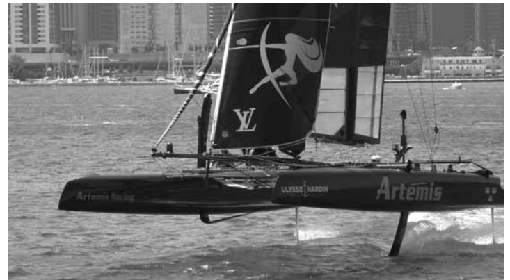
Photos from Louis Vuitton America's Cup World Series Chicago: Top, Groupama Team France (FRA) on the crane hoist during launch, above, Artemis Racing (SWE) flying on dagger-board and T-rudder foils. (next LVACWS regatta is July 23-24 in Portsmouth, UK).
